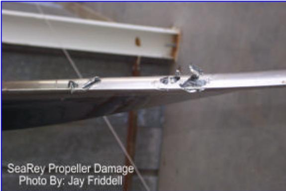
Fortunately, the damage was slight. A phone call to Ivoprop, the propeller manufacturer, established that I need only to fill any nicks with resin, reshape and smooth the damaged area, then install a new stainless steel tape. Of course, this could have been much worse! The propeller could have driven the cap through the fuselage, a tail surface, or possibly, through one of the flaps. The only significant expense, was a new radiator cap – would you believe \$52?
