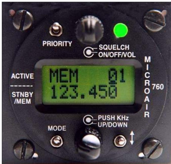
Mounting is into a standard 2¼" instrument hole and it runs on a 12-volt system. It weighs only 17 ounces, so it needs no additional support like some tray-mount radios and is very easy on the weight-and-balance sheet. I replaced a Collins professional comm, which sat in a ½-width radio tray, so I needed to make an adapter for my Kitfox panel with a 2¼" hole in it. My aircraft lost over two pounds when I made the swap.
